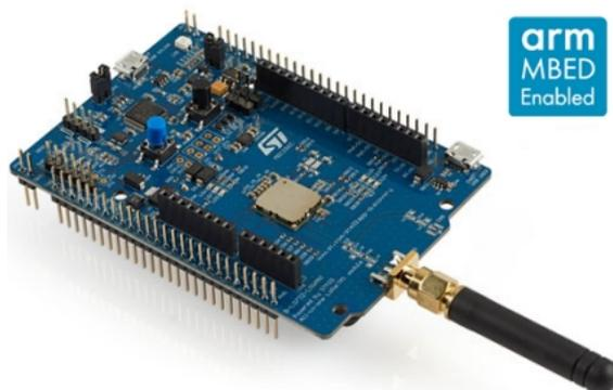
Figure 136: ST B-L072Z-LRWAN1 Discovery Board
