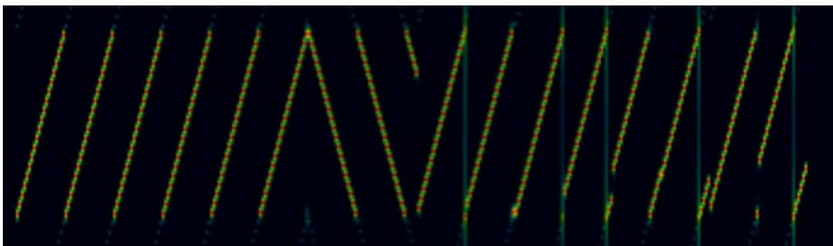
Figure 13: Spectrogram of a LoRa transmission
