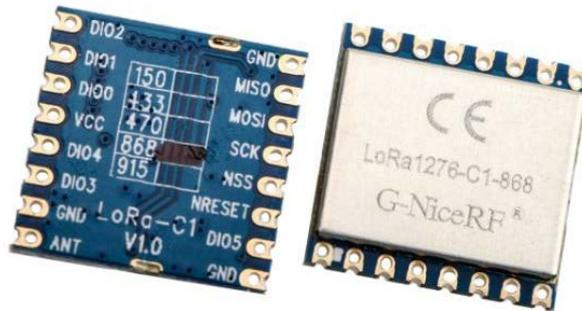
Figure 132: Example of a transceiver module (NiceRF)
