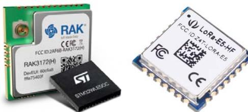
Figure 142: RAK3172 (left) and LoRa-E5 (right)
