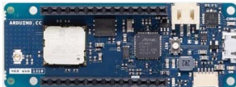
Figure 139: Arduino MKRWAN 1310: ATMEGA 32 bits microcontroller + CMWX1ZZABZ Module
